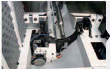
On-board sharpening operations usually take a long time and must be performed by experts. To make these operations simple, fast and precise, on Topset Master the stone automatically moves both axially and radially thanks to an electronic system with speed that can be preset depending on the type of stone/tool and stock removal.
