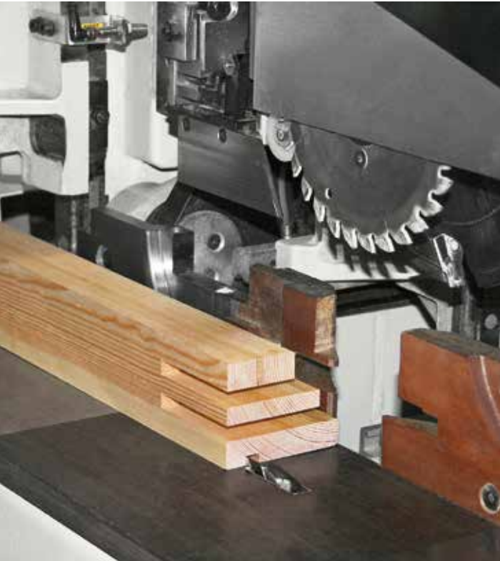
Horizontal unit for the machining of the bottom side of the work-piece.
