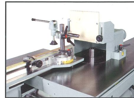
CUFFIA TOUPIE PER LAVORAZIONE DI TENONATURA – MOULDING FENCE FOR TENONING WORKS
