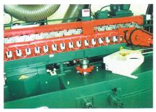
Bottom and top planer shaft with precision spindle bearings and at 30° angle, for perfect surfaces without hits / steps.
