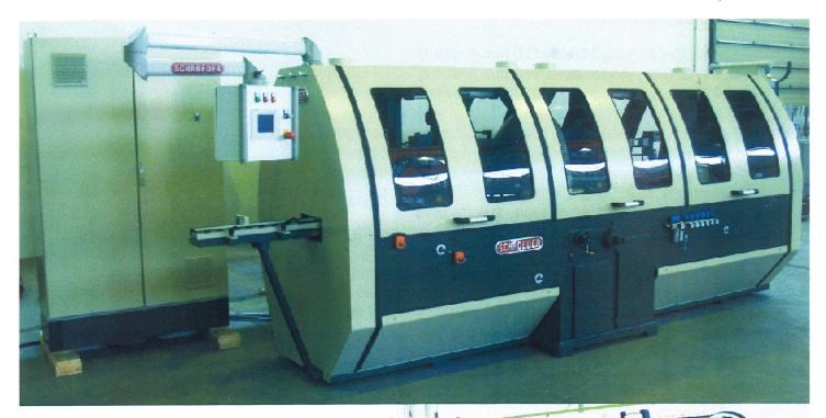
4-side planer for high precision (solid parquet and top layer blocks) and high capacity applications (feed speed 15 - 50 m/min.), specially designed for short wood blocks from 200 mm min. length.
