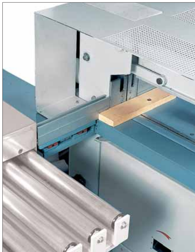
Botola espulsione rifili e scarti (aperta) Trap door for trim and waste ejection (open)
