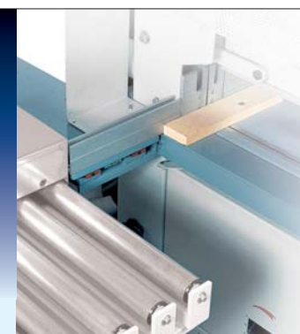
Botola espulsione rifili e scarti (aperta) Trap door for trim and waste ejection (open)
