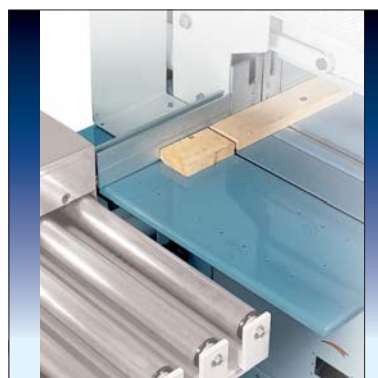
Botola espulsione rifili e scarti (chiusa) Trap door for trim and waste ejection (close)
