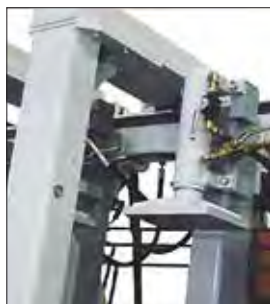
Cylinders and pressure clamps fitted with independent open/close valve.
