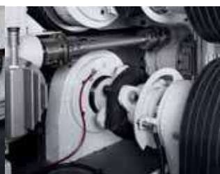
Rubber coupling Vibration-absorbing rubber coupling for contact drum.
