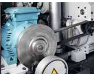
Feed drive with worm gear Direct power transmission and very constant torque with a large speed range.
