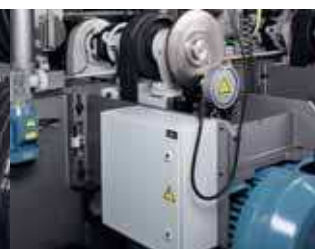
Main drive system For contact drum with disk brake for less vibration and optimised access to V-belt.
