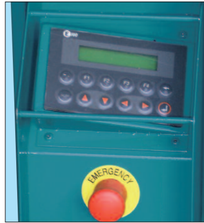
HMI Control Unit
