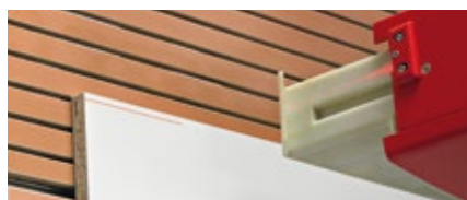
Laser-assisted indication of the horizontal cut (standard)
