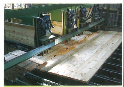
Each layer is automatically stacked using a backstop which holds back the last workpiece in the layer ensuring a very neat and reliable stacking.
