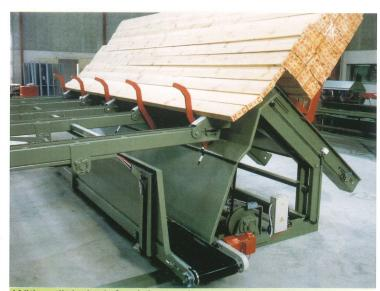
With a tilt hoist infeed the cutting capacity can be greatly increased. For the safe and careful handling, the tilt hoist can be equipped with hold back arms, ensuring gentle and well-controlled descent onto the cross chain conveyor, reducing noise and damage to the timber or chains.
