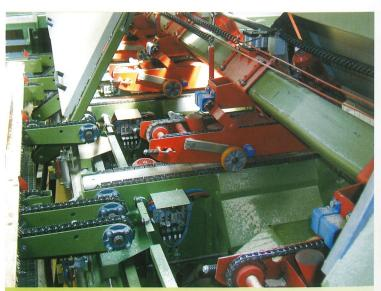
A multiple cross cut system can be equipped with up to eight saw units. Each unit can be either manually, electronically or CNC adjustable. The saw units are suspended on a height adjustable gantry so that all units can be set at a time.
