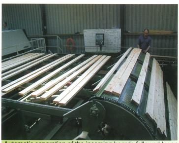
Automatic separation of the incoming boards followed by an automatic fair-ending of the boards ensuring a fast and continous infeed to the saw.
