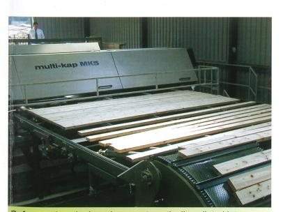
Before cutting, the boards are automatically collated into layers and, in one movement, efficiently fed into the saw.
