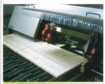
After cutting the boards are automatically and reliably stacked into layers.
