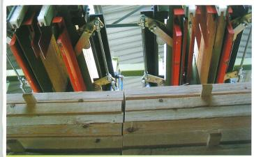
Stability sticks can be placed between a requested number of layers ensuring high stability and transportability of timber packs.
