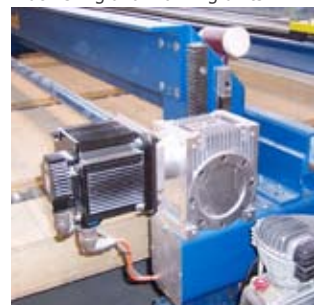
large gantry-motor to generate the pressure of the serrage
