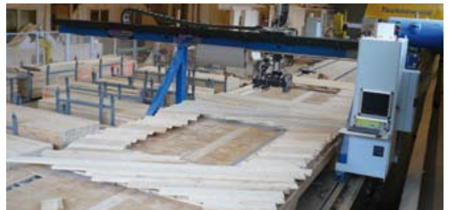
wall element with large window opening
