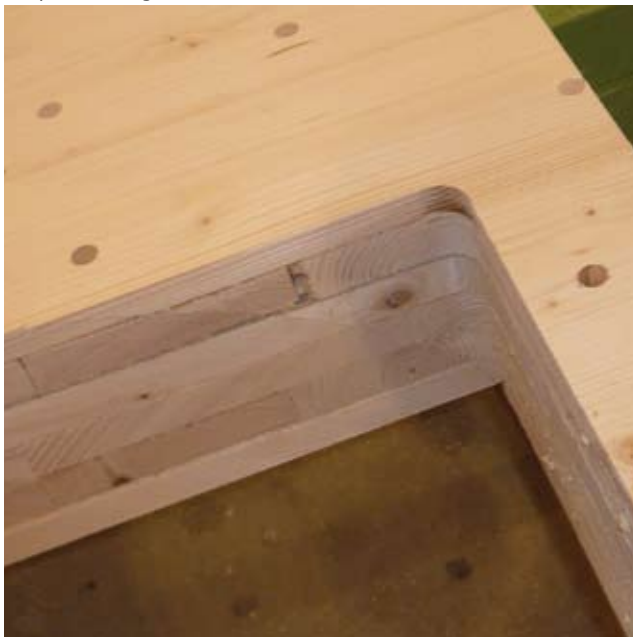
window opening with saw and finger shaper
