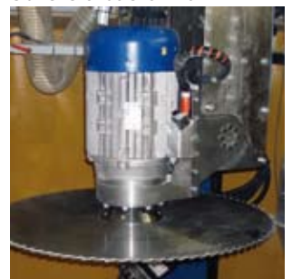
flangeless saw can be swivelled for up to 92°
