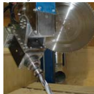
water-cooled high-performance spindle with HSK tool holder
