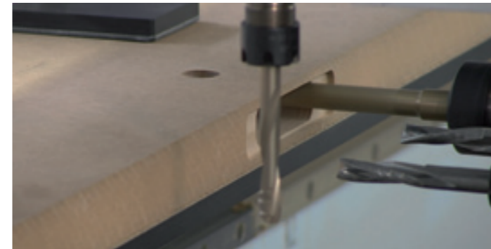
Processing of lock-case and handle/keyhole
