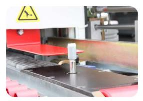
One of the most significant features of this machine is pneumatic stop system.
