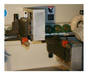
**Top & Bottom straight Scraper Unit** cleans the top and bottom excessive band and provides better finish on the workpiece.
