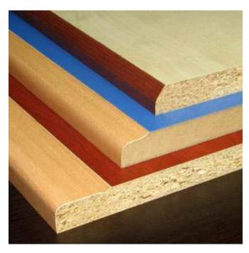
SOME SAMPLE WORKPIECES ( CHIPBOARD & MDF) PROCESSED IN SOFTFORMING MACHINE.
