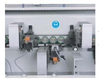
**Top & Bottom Trimming Unit**. Contains 2 high frequency 12.000 rpm Italian made motors to guarantee the best possibile and cleanest result.
