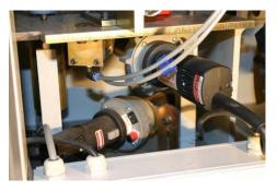
**Hot Air Blower** applies heat to the pre-glued band to activate the glue.
