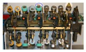
**Triple Cartridge Group.** Applies the band to the profiled edges by the use of rollers arranged in an appropriate way. Three profiles are already included in the machine. It is very simple to interchange between the profiles.
