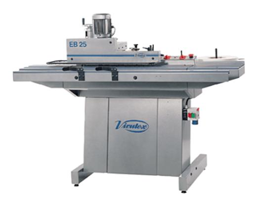
For panel edgebanding with preglued PVC, melamine and veneer. Automatic edge feeding system. Trimming on both sides. Motorized top and bottom trimming unit. Front edge trimming, rear flush cutting of the tape. No compressed air or dust collector required. Powerful hot air system with electronic temperature control. Minimum heat up time (2min.). Belt feeder for automatic workpiece.
