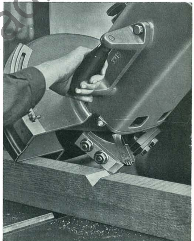
Shows the machine canted for such work as birdsmouthing in roof spars.
