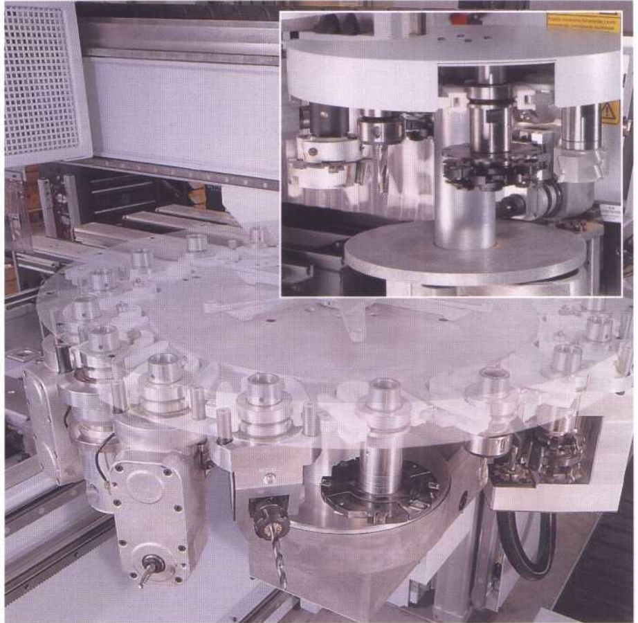
8- or 18-position magazine with X-axis ride along
