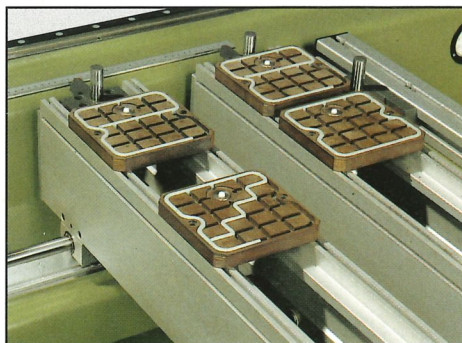
Suction cups with variable suction area for easy contouring.
