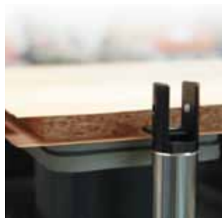
Tilting stops for veneer overhang Guarantee simple positioning of panels with veneer overhang
