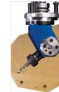
Drilling/Routing, swivelling cranked – (0° - 90°)
