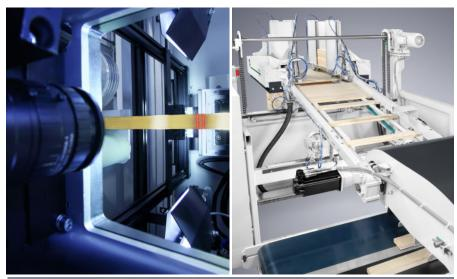
**WEINIG Scanner systems** detect fully automatically and at lightning speed relevant workpiece characteristics such as branches, cracks and structural patterns, and supply up to 4 OptiCut high-speed saws with cutting data via intelligent mechanisms while maintaining full production speed.
