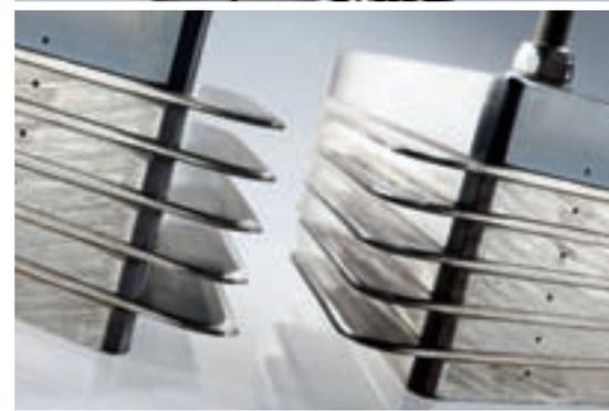
**Splitting unit** – Profitable production of lamellas requires process reliability, short setup times and maximum wood yield. The Powermat satisfies these requirements ideally: The wood can be processed in one workstep; first by planing all 4 sides and then ripping. Resulting in high production capability. During this process the material is pressed flat against the guiding surfaces, resulting in significant savings in material.
