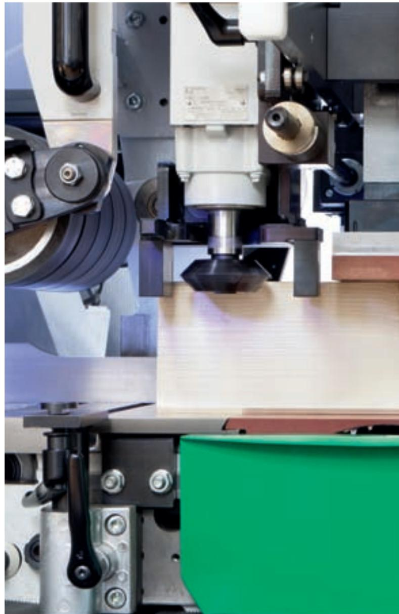
exceptional rigidity of the PowerLock HSK tool system and controlled guidance of the workpiece across the full width provide ideal conditions for perfect processing of large wood pieces.
