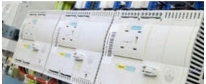
The high tech electrics in our moulders are developed in close cooperation with international companies such as Siemens. For example, the new motor starter design resets its parameters according to the weight of a newly inserted tool and optimizes the load.
