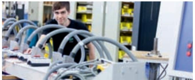
A faulty contact in the electrical system can cause the machine to shut down. WEINIG switch cabinets undergo a comprehensive functional test according to a checklist before leaving the assembly area. All working processes of the moulder are simulated.
