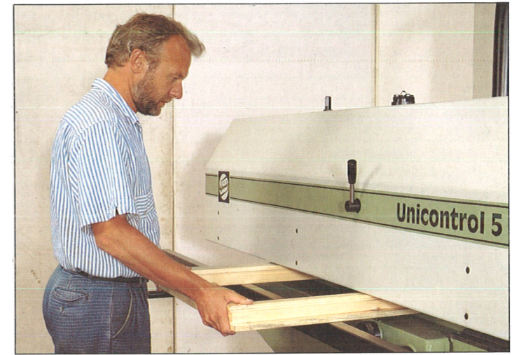
Stormproofing of window sashes – precise and without any tear-out.
