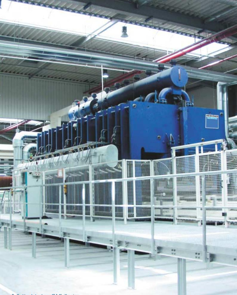
The Wemhöner short-cycle press KT-F-1E with maximum: Press surface of 13.0 meters in length and 2.7 meters in width, 600 N/cm<sup>2</sup> specific pressure, 220 degrees heating plate temperature and 225 cycles per hour.
