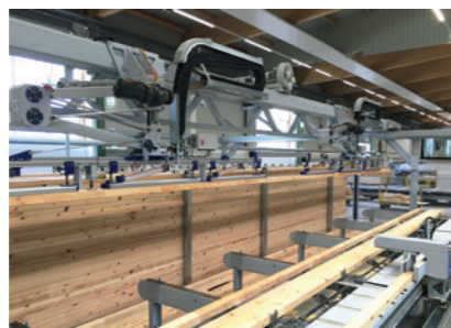
Powerful and flexible Processing system with feeding portal and integrated storage
