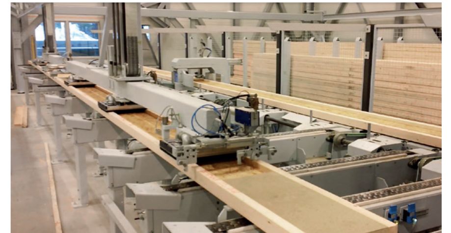
Versatile stud feeding Handling portal for stud feeding with integrated sorting unit
