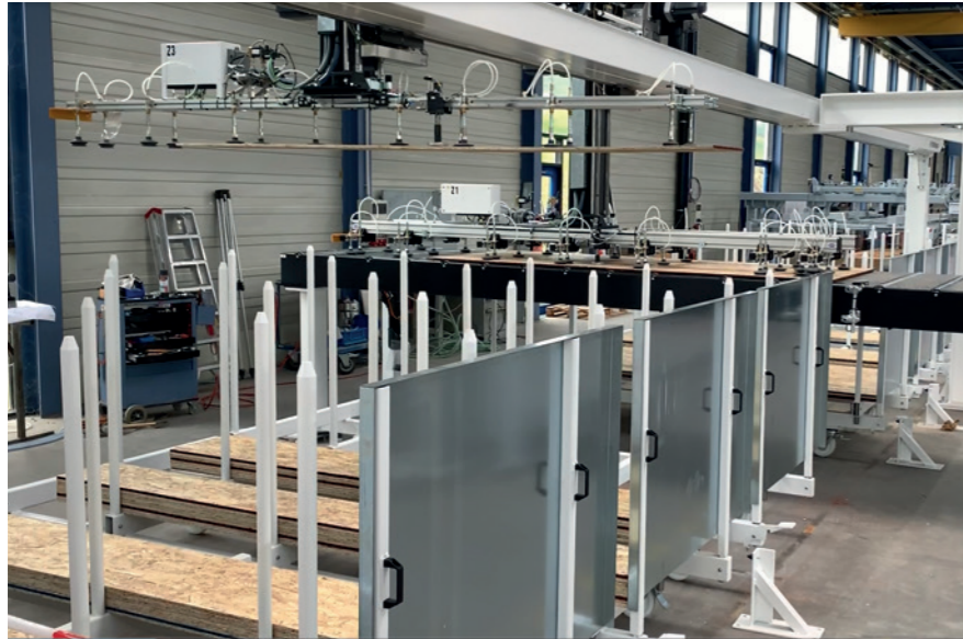
Efficient panel handling Fully automatic feeding portal for panel materials
