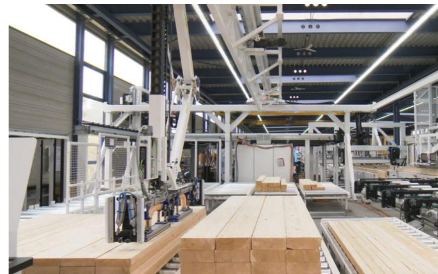
Versatile stud feeding Handling portal for stud feeding with integrated sorting unit
