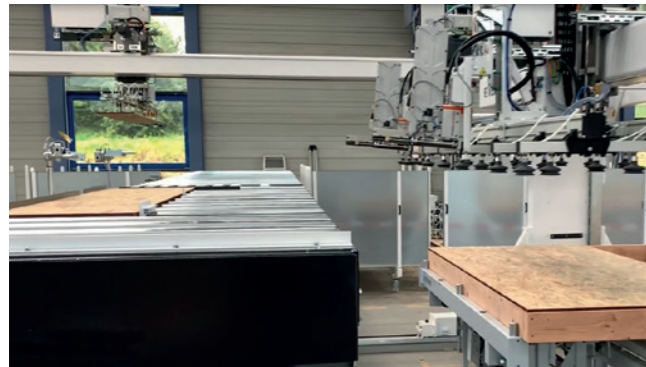
Just-in-time stud feeding Framework station with integrated feeding portal for six stud cross-sections
