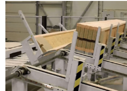
Material handling and processing in stacks Material feed with automatic stacking for efficient cutting
