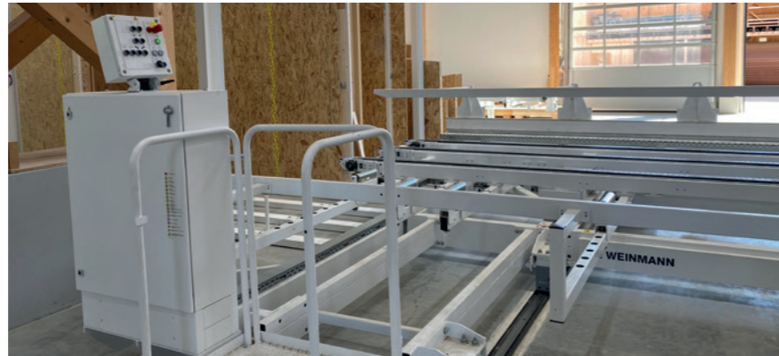
Traveling operator podium
