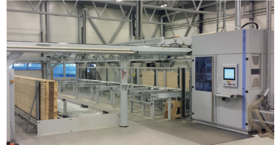
Material handling and processing in stacks Material feed with automatic stacking for efficient cutting
