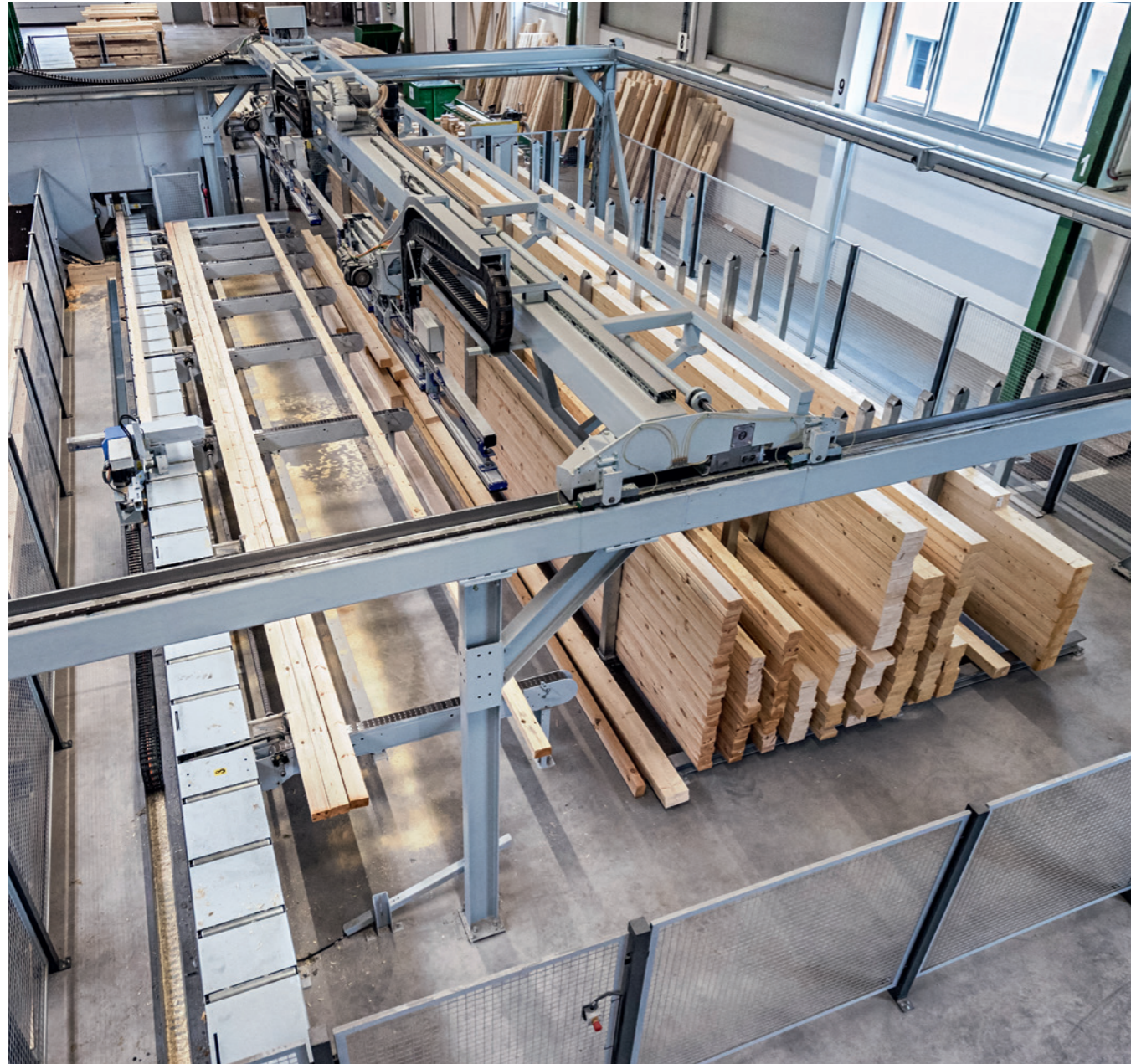
Powerful and flexible Processing system with feeding portal and integrated storage
