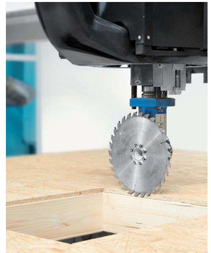
Manufacturing window openings
