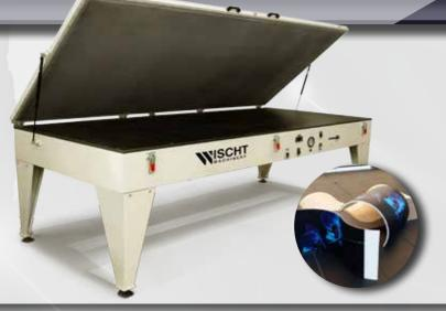
With WISCHT COLD PRESS in combination with an heating oven or WISCHT WPE-Subli machine, you can make high quality thermoforming process. Thermoforming is a manufacturing process where a plastic sheet is heated to a pliable forming temperature, formed to a specific shape in a mold, and trimmed to create a usable product.
