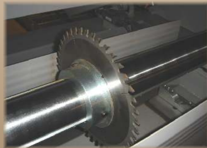
Mechanical-lock tool holder bush (on request)
