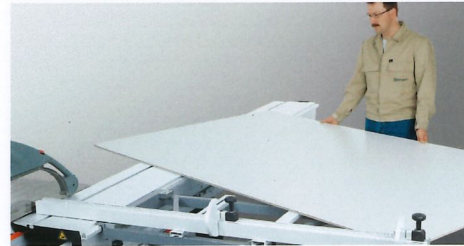
2. Turn the panel anti-clockwise and place the trimmed edge against the fence.
