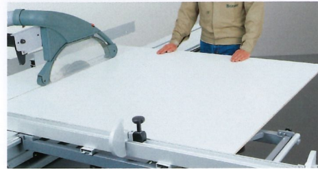
2. Cut panel strips on the rip fence.
