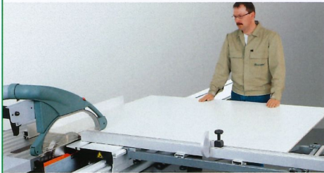
1. Position the rip fence in front of the saw blade and set the width.
