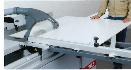
3. Cut the remaining piece to width on the crosscut fence.
