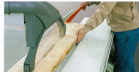
3. Guide the workpiece along the rip fence and through the rotating saw blade, using the push stick if necessary.
