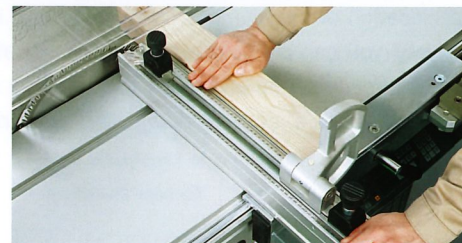
3. Cut the remaining piece to size on the crosscut fence.
