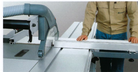
2. Cut panel strip to final length on the rip fence.
