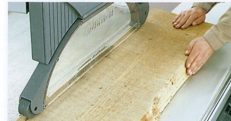
3. Guide the workpiece safely through the rotating saw blade on the sliding table.
