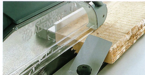
2. The clamping shoe secures the board on the sliding table.
