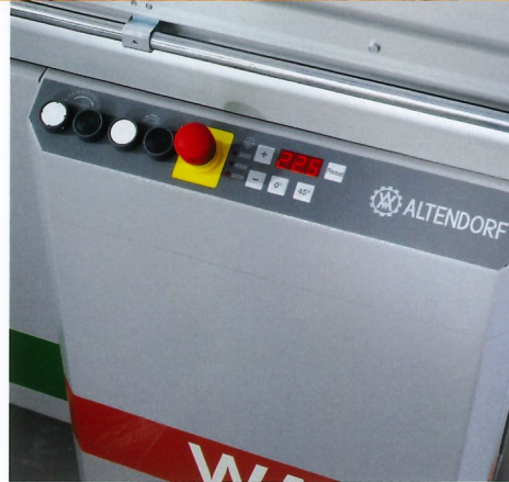
Motorised rise/fall and tilt adjustment of the saw blade.
