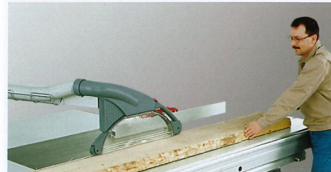
2. Align and trim the material along the cutting line.
