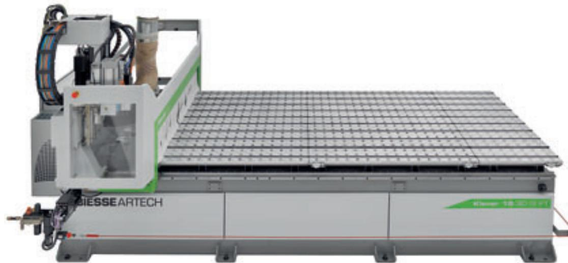
Aluminium working table with vacuum system: allows manual locking using T slots or vacuum locking (optional).
