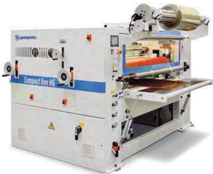
Single sided compact laminating machine with smoothing roller suitable for the application of glue on transparent foil and overlay it afterwards on melamine coated or digital printed panels achieving a bright high gloss finish. Any other type of foil can be applied obtaining the highest finishing quality as well.
