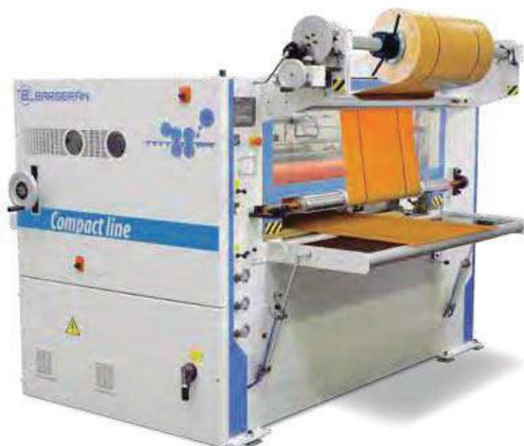
Single sided compact laminating machine for the application of paper foil, PVC and low pressure laminates (CPL) on panels made of MDF or particleboard using EVA or PUR hotmelt glues.
