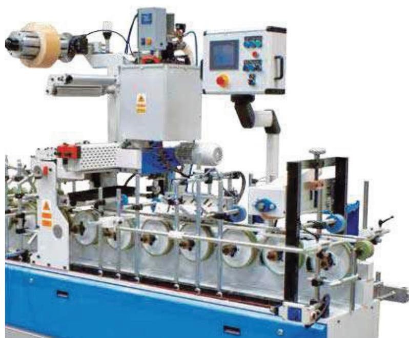
Profile wrapping machine designed for the gluing and application of rolled material on profiles, made of MDF, particleboard, low quality wood, etc. by means of a slot nozzle head for EVA hot melt glue.
