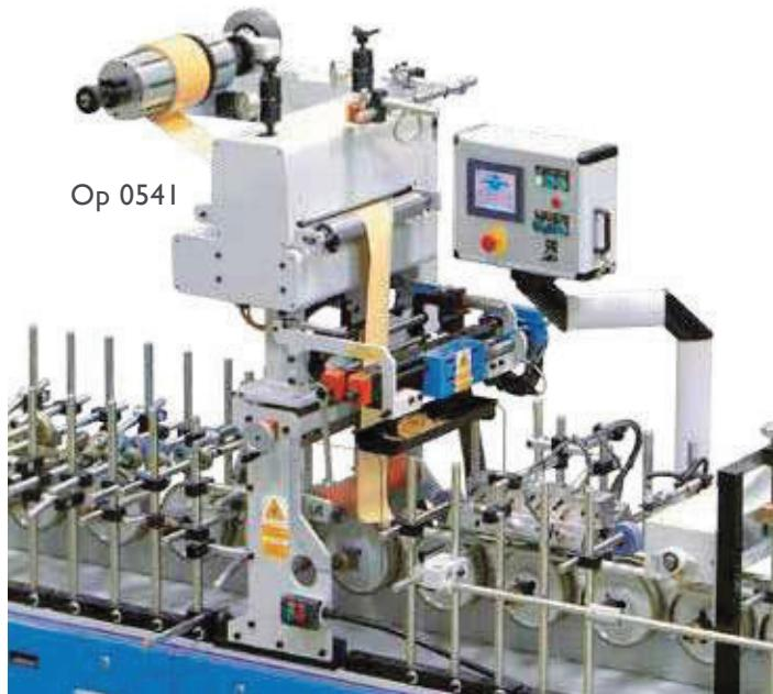
Pre-cutting system for wooden veneer, paper and PVC foils, low pressure laminates and similar materials from the roll, so that the profiles can be separated at the machine's outfeed.
