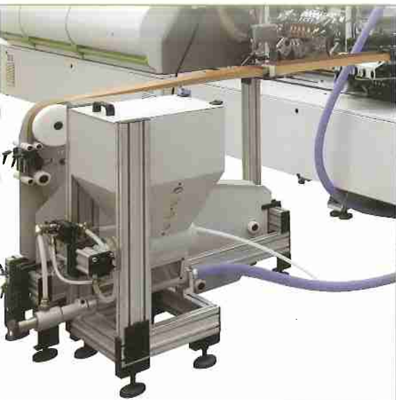
Glue tank feeder from ground
