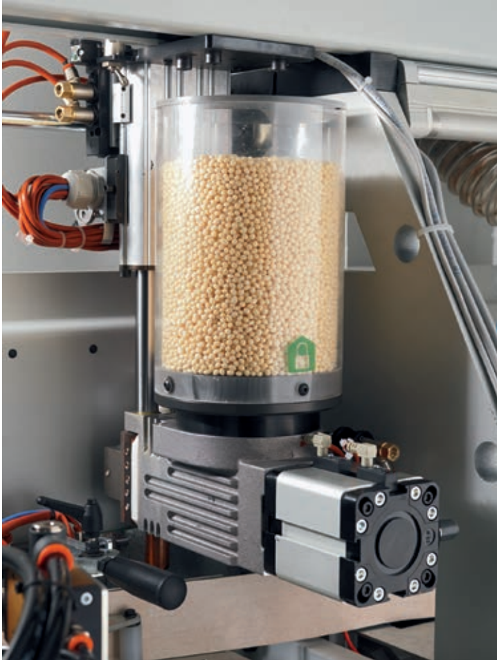
Pre-melting system for EVA glue.
