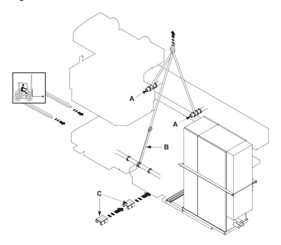
To unload the main structure, hook the lifting cables to the two round bars A and to bracket B.
