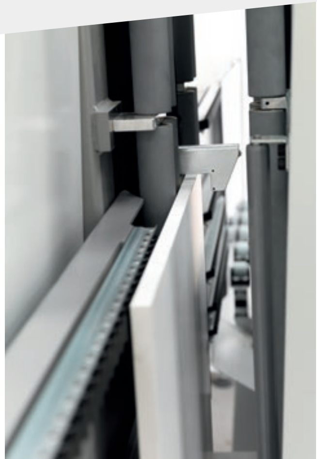
The upper sensor systems consists of two photocells that can detect the panel's height and correct the size with respect to the "Y" axis.
