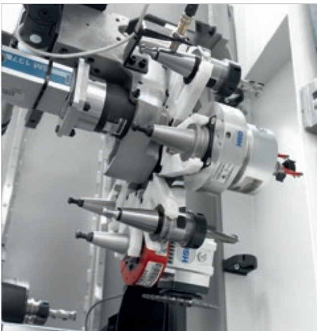
8-position tool magazine that manages different types of aggregates, thus increasing the machine's versatility.
