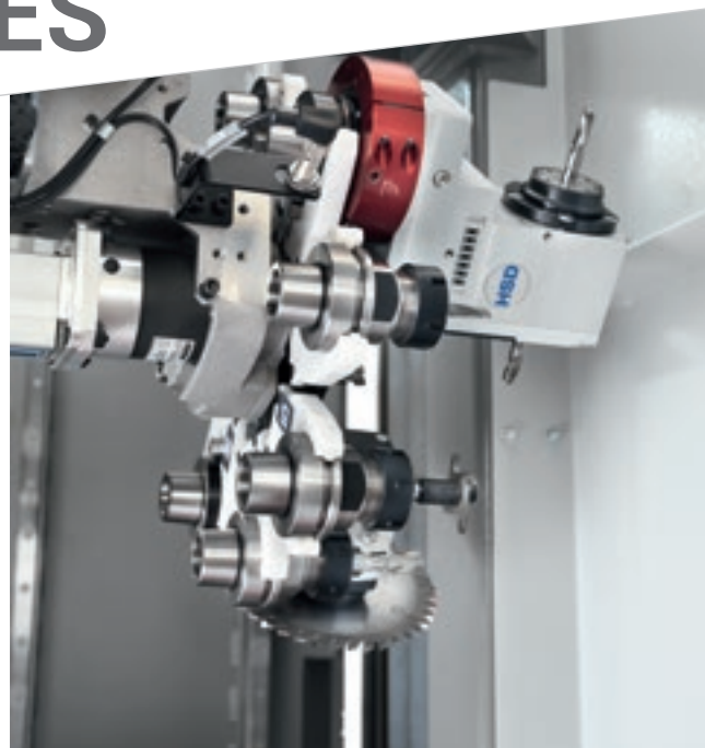
8-position tool magazine that manages different types of aggregates, thus increasing the machine's versatility.
