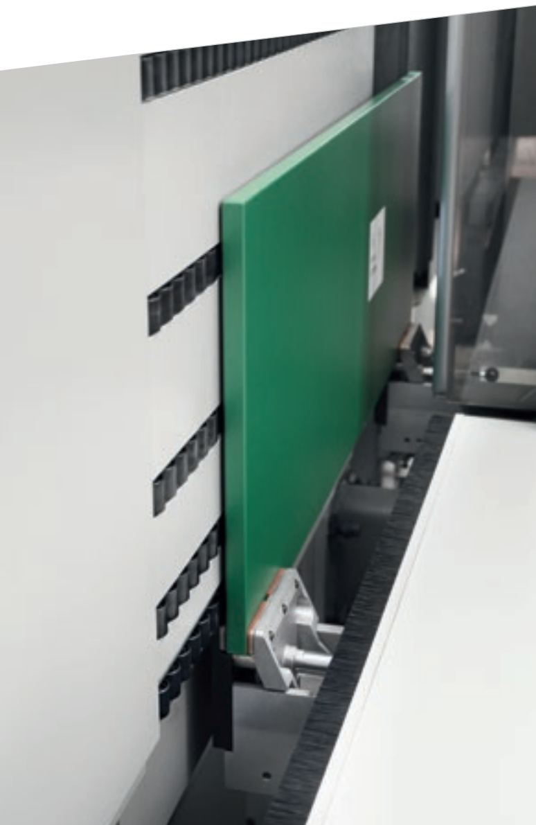
8-position tool magazine that manages different types of aggregates, thus increasing the machine's versatility.
