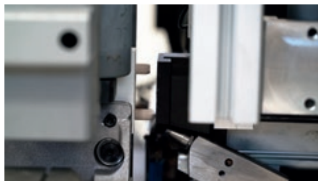
Unit for managing glue/dowel insertion with a patented system with tool change for recalling the work aggregate.
