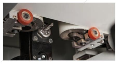
Patented dual-section haul-off for machining the 4 panel edges without limits (not available on Vektor 25 and 30).
