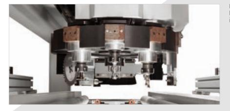
Revolver "R10" unit with tool change in less than 2 seconds, during the machining operation.
