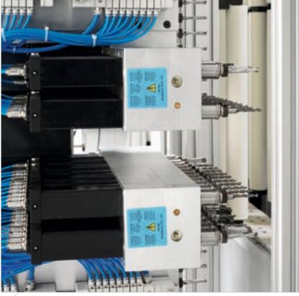
Unit with independent spindles for personalised boring operations.
