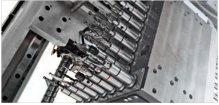
Work units that help optimise the process, reducing the number of boring descents and therefore the overall machining times.
