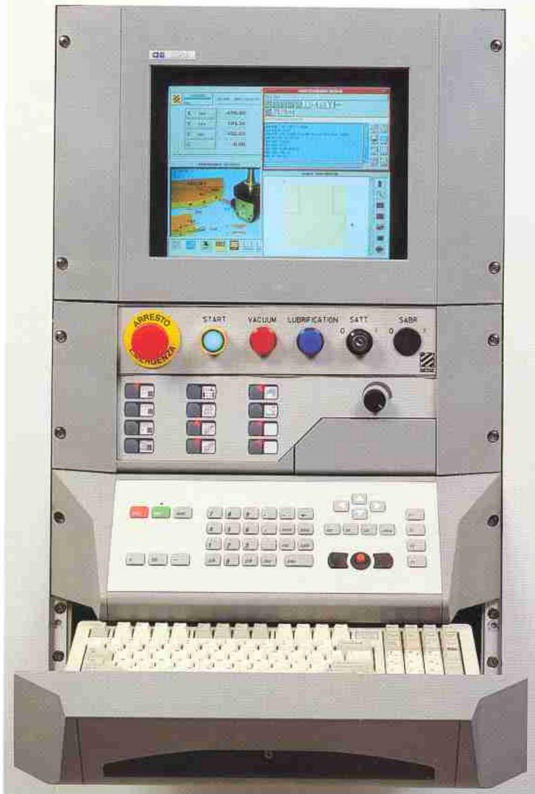
The Numerical Control XNC is equipped with two keyboards, one industrial keyboard IP 65 with mouse included and the second a standard P.C. keyboard situated in a dust free enclosure.
