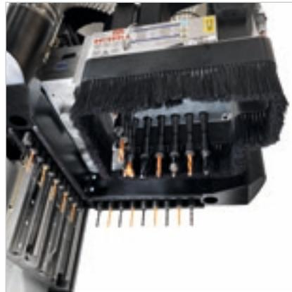
The new additional **OddBits boring head**, combined with a BH20, is a second boring head with independently removable spindles and a dedicated motor. The head is particularly useful for nest-based machining operations where panels are positioned in the nest with a 90° step rotation.
