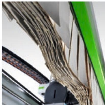
22 overlaid layers of **side curtain guards** to protect the working unit, which are movable to enable the machine to work at maximum speed in total safety.
