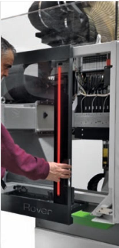
Long term safety and reliability thanks to the new **bumpers** combined with **photocells** with no footprint or mechanical wear.
