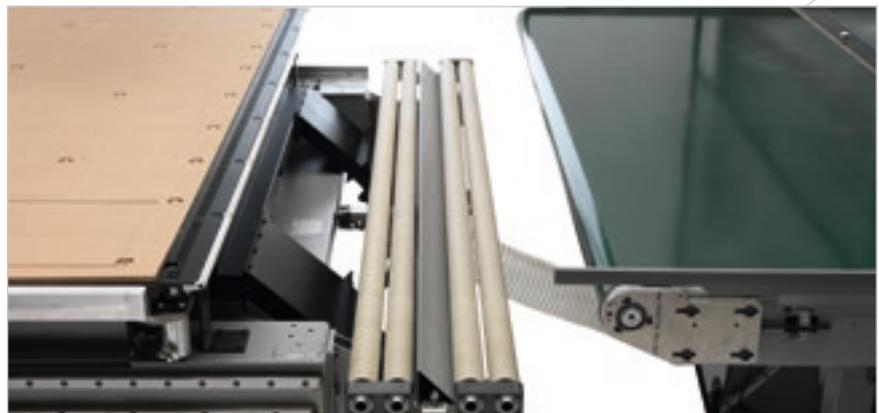
The **loop presser** supports the machining of curved and stacked panels by applying pressure to the upper surface of the panel.
