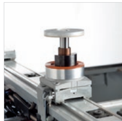
Hyperclamp for rigid and precise locking.
