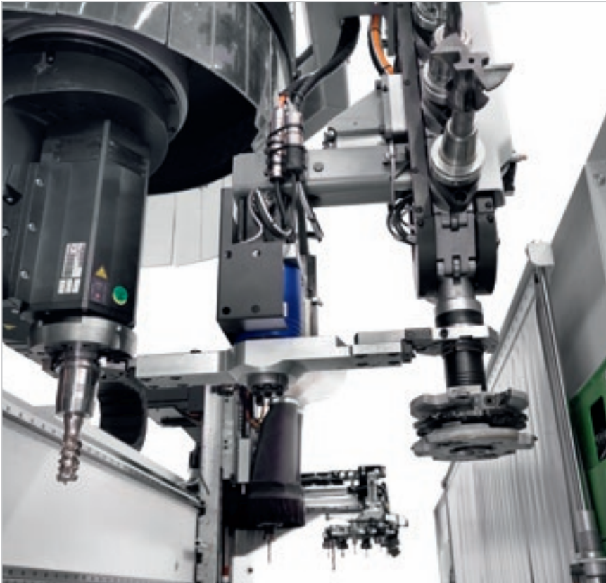
Vertical chain tool magazine on Y axis with 10-15 positions.
