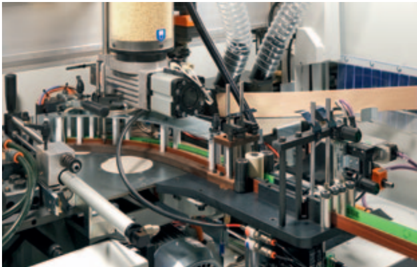
Automatic edge changement, managed by PC-Flat (opt).
