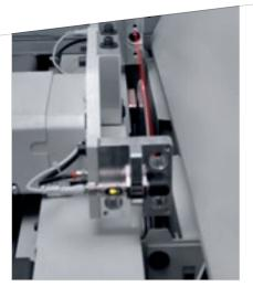
Automatic alignment. The patented system automatically aligns the scoring blade in seconds, which completely eliminates test cuts, reduces set-up time which increases efficiency and reduces production costs.
