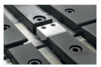
Cutting line closure system, to prevent the longitudinal trim cuts from falling into the machine and fouling the blade path.
