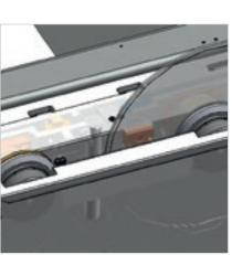
The anti-slide device controls the blade position and number of rotations, intervening to adjust the advance speed. Maximum cutting quality, a longer blade lifespan, and reduced maintenance costs.
