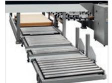
Infeed conveyors with free-running or powered rollers allow the loading and side or rear unloading of the panels.
