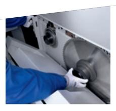
The "Quick change" system is the **fast-est, safest and most ergonomic** device for replacing the blades without using tools.
