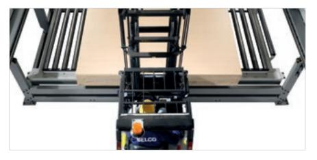
The lift table consists of a strong frame and is equipped with a special structure to load the pack of panels directly by forklift.
