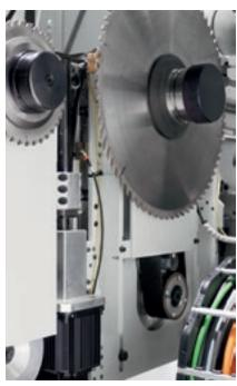
The motorised vertical blade adjustment ensures **precise**, **quick adjustment** of blade protrusion.
