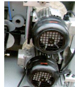
**Brushing Unit** To carry out the cleaning and polishing of the applied edge using cloth disc brushes with 2 motors 0.25 hp (0.18 kW) with cloth discs dia. 3.8" / 100 mm.
