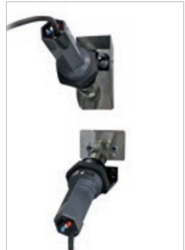
Hot air blower for reactivating the color of the edges.
