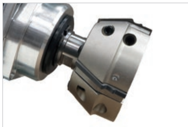
Multi-profile tools for various types of edgebanding strip.
