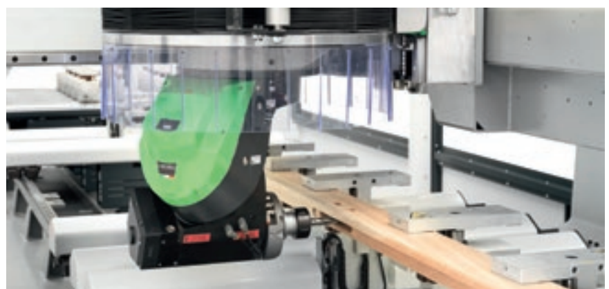
A 16.5 kW 5-axis head aimed at the hardwood: powerful and sturdy for laborious cutting.
