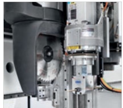
Electrospindle, 19.2 kW. FlexyWood PLUS. Unit 3+1.
