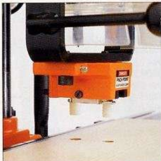
press-in plate installation
