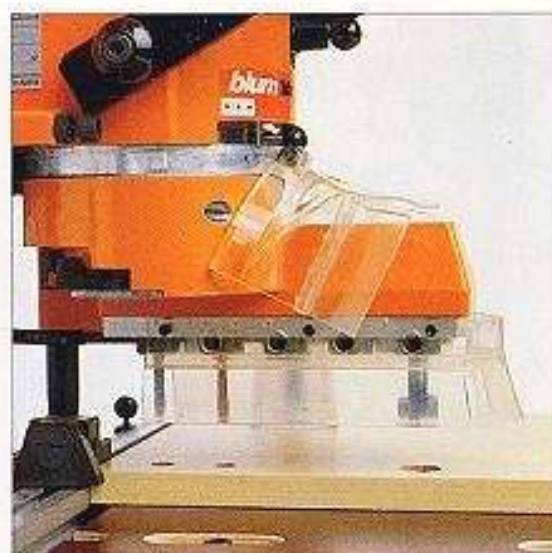
drilling mounting holes
