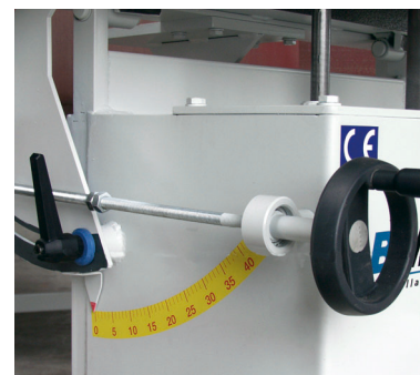
Graduation and hand wheel for adjusting the sanding unit under an angle
