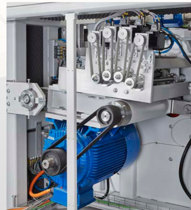
Sawblades positioning with Brushless motors
