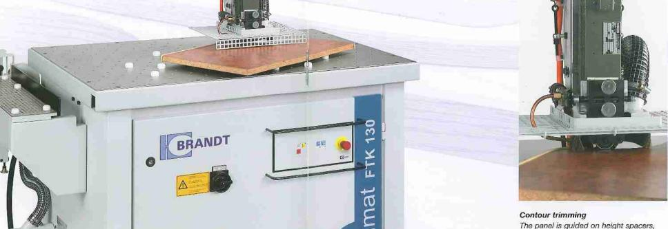
which are fixed on the working tabel according to workpiece shape.
